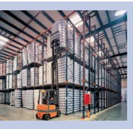
**Drive-In/Drive-Thru.** With drive-in or drive-thru pallet rack, product is stored within lanes several pallets deep. Lift trucks place the pallets on supporting rails connected to the upright frames.
