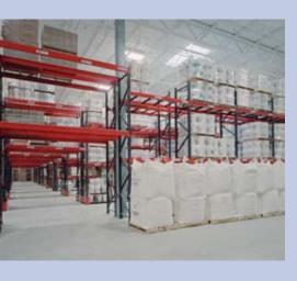
**Selective Rack.** Combining vertical frames with horizontal load beams, single-depth selective pallet rack provides total accessibility to the product. Easily the most popular racking system in use today, it provides the versatility required for warehouses that have a wide variety of product types. Storage density is compromised due to this flexibility, in addition to the fact that the aisles must be wide enough for fork trucks to maneuver.
