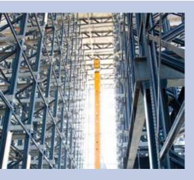
**Unit Load AS/RS.** Created to meet the need for maximizing available vertical space while maintaining a compact footprint, the unit load AS/RS can save up to 40% of storage space over conventional storage solutions. This system fully automates the entry and exit of goods and provides total control over product inventory. High-speed stacker cranes move within very narrow aisles and can reach heights of nearly 100 feet when retrieving or depositing a load.
