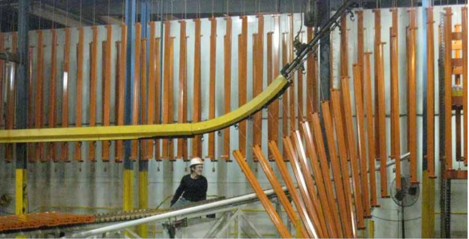
*PAINT WASTING TIME, NO MORE: Steel beams sprayed along the line in the powder coating process leave a lot of wasted paint in between each beam. The Interlake Mecalux Plant in South Carolina has continually found ways to minimize such waste.*
