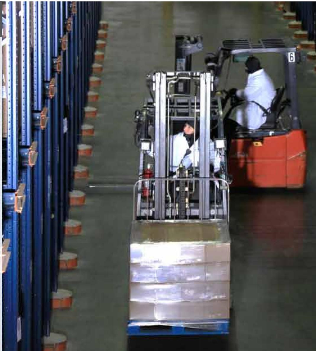
*OPPOSITE: Blencor uses special lift trucks capable of reaching advanced heights and handling double-pallet weight. THIS PAGE: Cement guard rails add extra protection against lift truck damage.*
