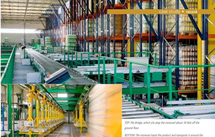
BOTTOM: The monorail loads the product and transports it around the track to the unloading zone about 6 feet across the aisle.
