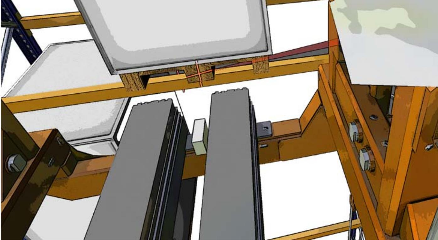
*ABOVE: Employing a combination of laser optics and cameras, a stacker crane adjusts its operations to make up for any type of deformation.*
