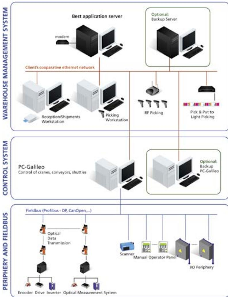
FIGURE 1: Total Control. Galileo plays a major part in parlaying communication with automated devices within a warehouse.
