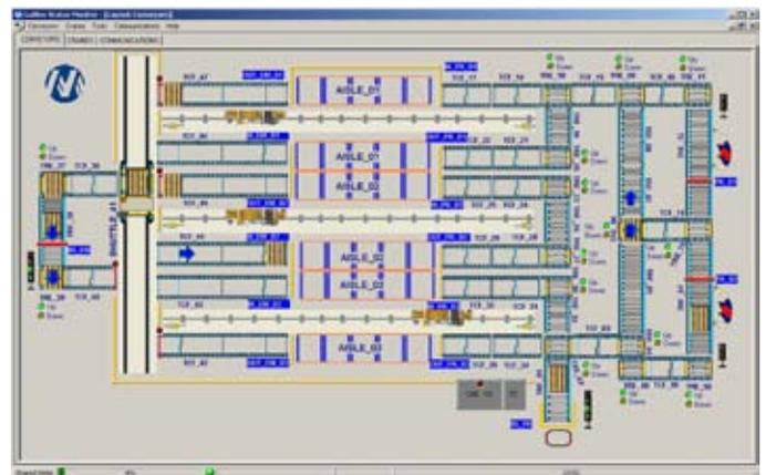
**Status Monitor** This is the Supervisory Control and Data Acquisition (SCADA) system monitor and problem diagnosis module that accounts for quality control of operations (Figure 4). The highly customizable Status Monitor provides a visual layout that allows operators to observe the function progress and locate any malfunction that may occur. This module allows warehouse operators to interact with facility operations and determine manual or automatic operations.
