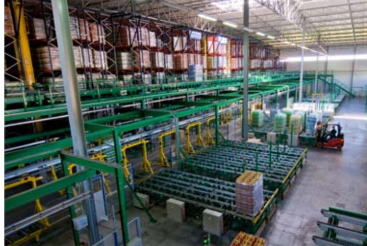
Load units which do not comply with the assumed criteria are instantly discarded onto another conveyor for correction
