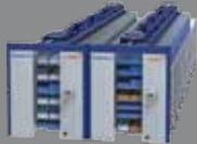
**Spinblock:** Automatic horizontal carousels, epitomizes the "product-to-man" concept by enabling a single worker to prepare up to 400 lanes alone.
