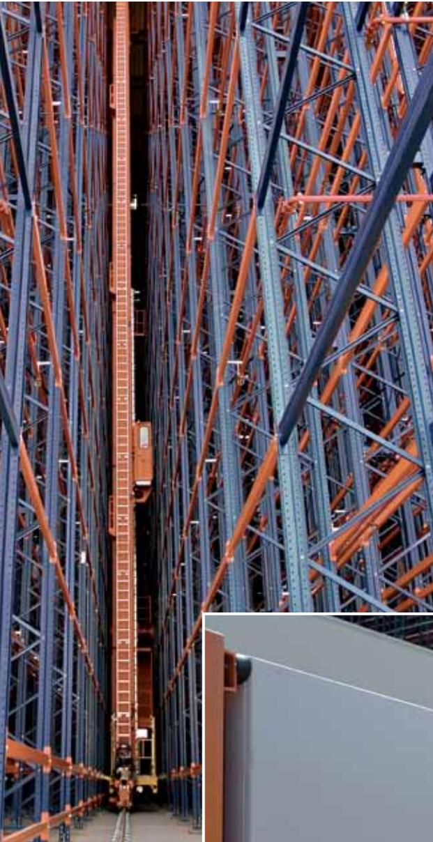
system to organize the stacker crane's motions. This times and coordinates the ascent and descent of the crane, making it use the least amount of energy, and the descent of one machine powers the ascent or startup of another.
