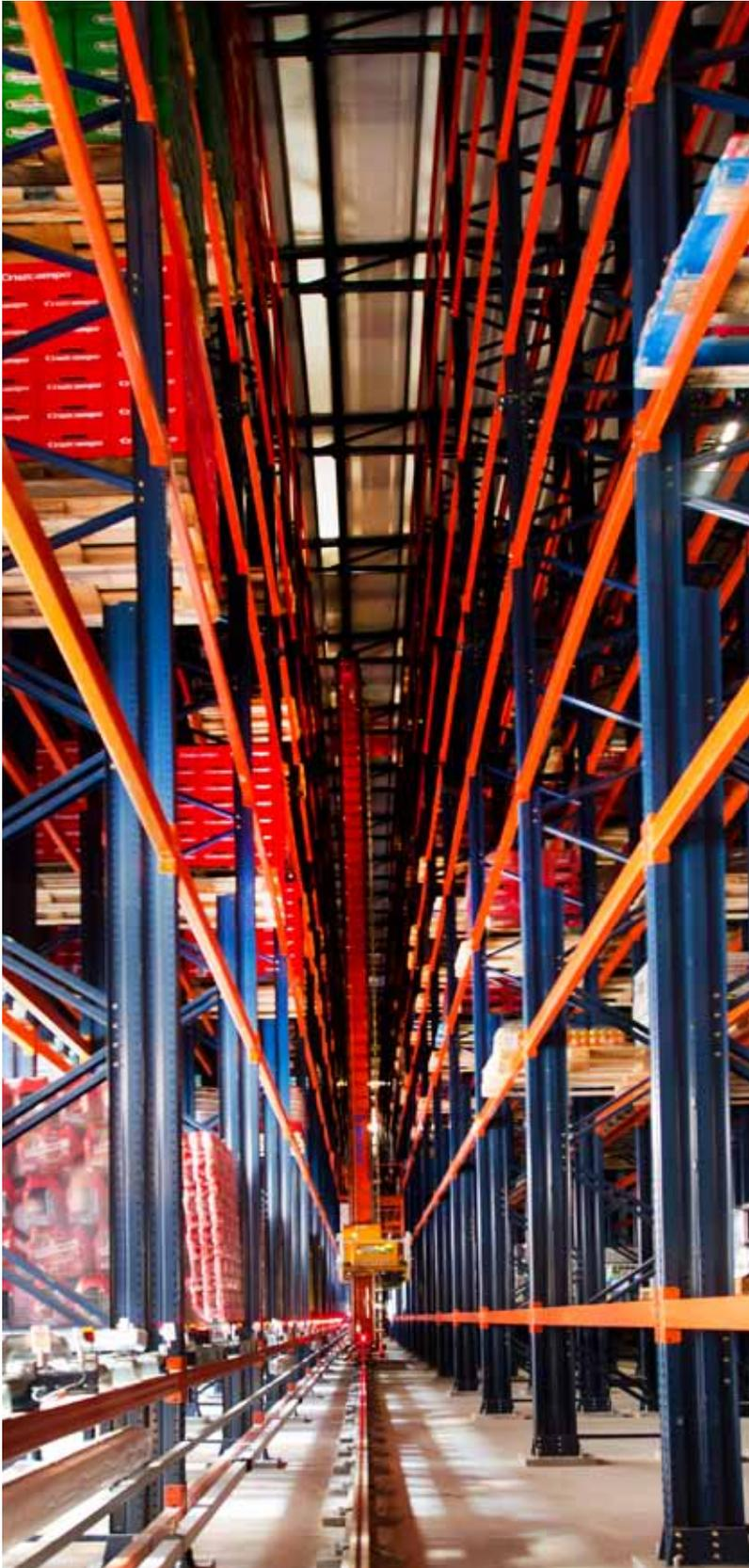
*By automating part of Amagosa's storage facility with narrow-aisle stacker cranes, the company was able to efficiently store and turnover more goods using less floor space for storage.*
