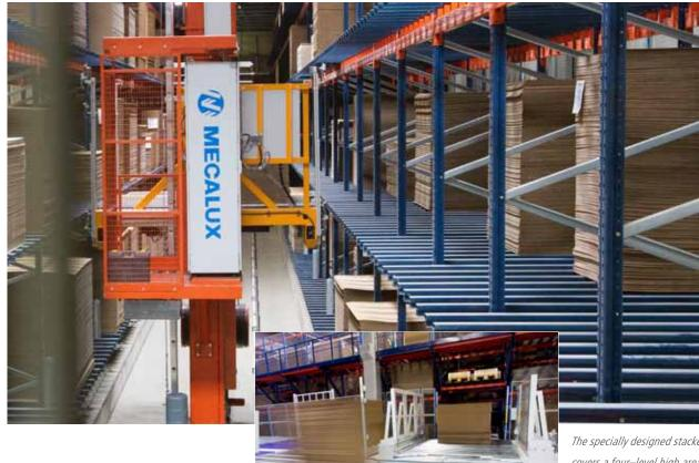
The specially designed stacker crane (top) covers a four-level high area and distributes goods that are then carried through a warehouse space almost 270 feet long.
