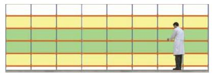
(TOP) A typical example of the inefficient footpath a poorly slotted warehouse may cause. (BOTTTOM) Vertical slotting is important, too. The higher turnover items should be placed in the green "sweetspot".
