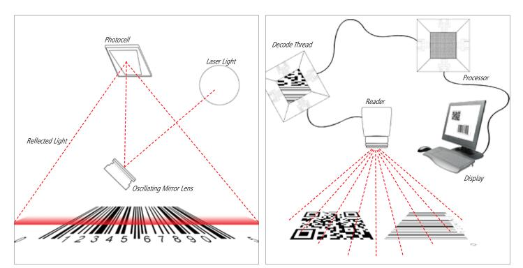
Figure 1: Illustration of a bar code scanner.
