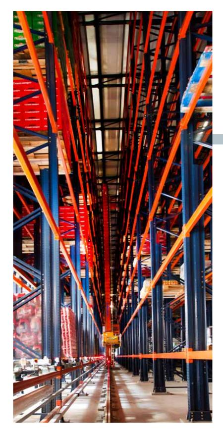
By automating part of Amagosa's storage facility with narrow—aisle stacker cranes, the company was able to efficiently store and turnover more goods using less floor space for storage.
