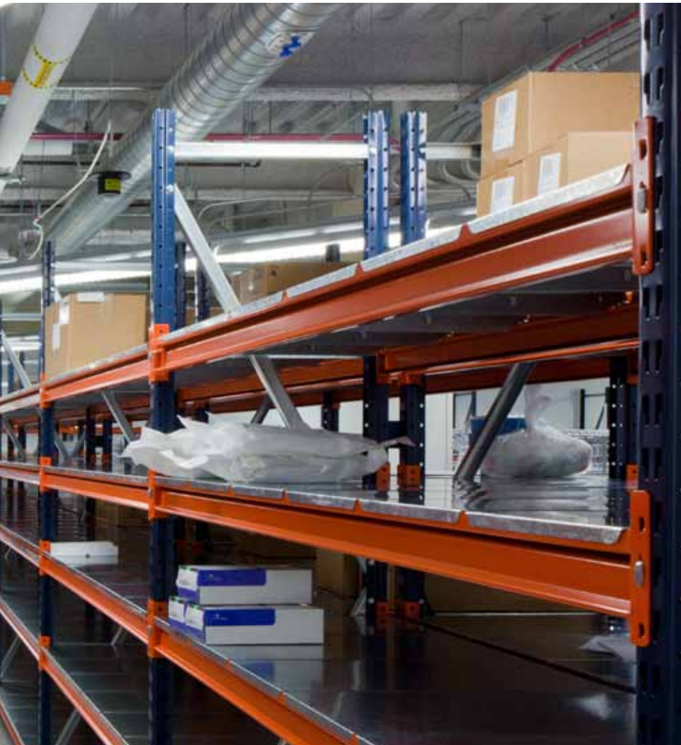
The galvanized steel shelving added to the rack allows for easier stacking and removal of simple handpicked goods, as there is less storage friction.
