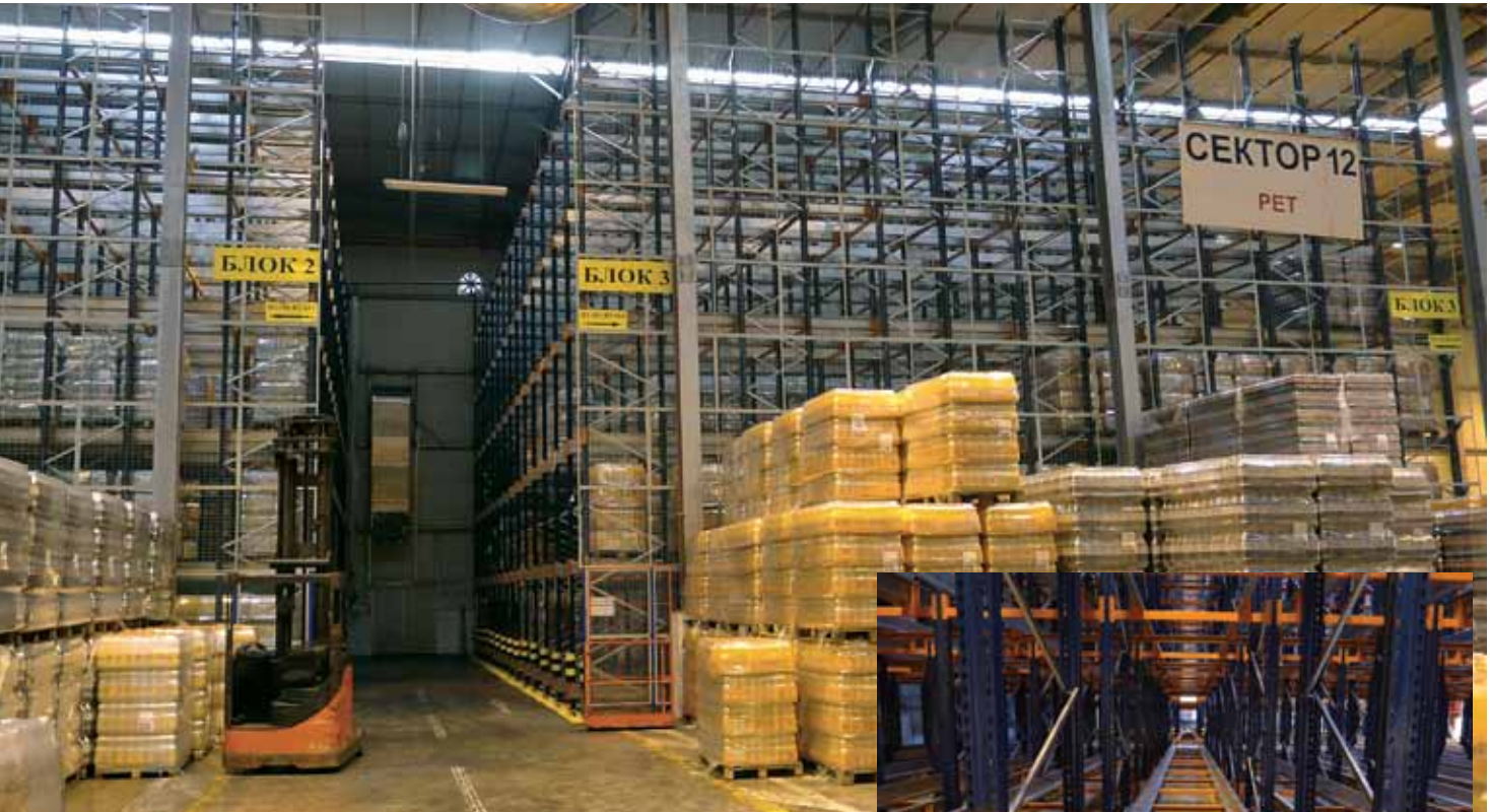
Above: Pallet Shuttle allows for a high-density, compact storage system. Right: A forklift sets the pallet on top of the Radio Shuttle, and the cart moves along the track to place the load in the correct location.
