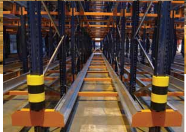
Above: Pallet Shuttle allows for a high-density, compact storage system. Right: A forklift sets the pallet on top of the Radio Shuttle, and the cart moves along the track to place the load in the correct location.
