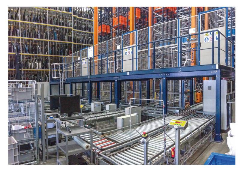
In merely 5.3% of the logistics center's total surface area, Zbeda Group has an automated warehouse that provides high throughput and streamlines order preparation locations each, 18 in total) equipped with put-to-light devices that help operators distribute the goods into various orders simultaneously. Once the product is received, the display lights up and shows the number of items the order requires, boosting efficiency and reducing possible errors.
