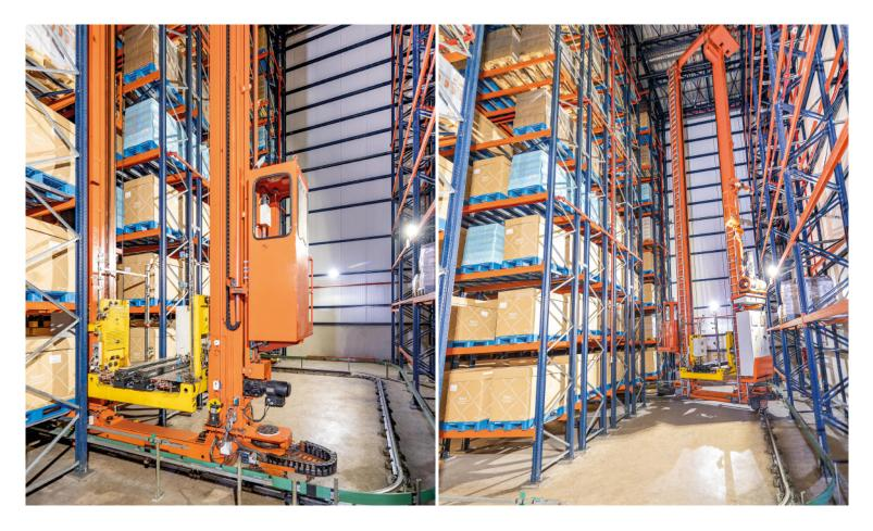
which operated in the three aisles. It did so by means of a system of curved rails set up at the back of the warehouse, enabling the stacker crane to change aisles as required. This solution is implemented when the storage volume is high and the flow of movements is moderate.
