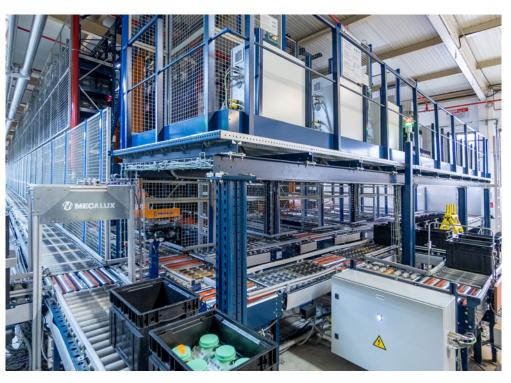
The AS/RS comprises three aisles with double-deep racking on each side. In this small space (the racks stand 13.1' high by 92' long), Schaeffler can store up to 490 different SKUs in 5,184 boxes measuring 15.6" x 11.7" with a maximum unit weight of 143.3 lb.
