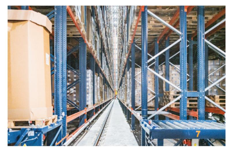
mizing the facility's floor space, this high-density storage and retrieval system (AS/RS) for 7,000 pallets has cut energy consumption; making better use of space reduces the volume of air to be cooled. Now, Saar has tripled its production pace, yielding up to 26,455 tons of deep-frozen vegetables annually.
