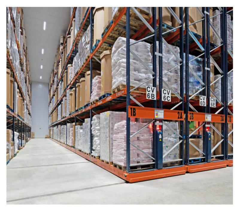
provides direct access to the goods. It does so by opening the required aisle by means of a remote control or directly via the onboard control panel.
