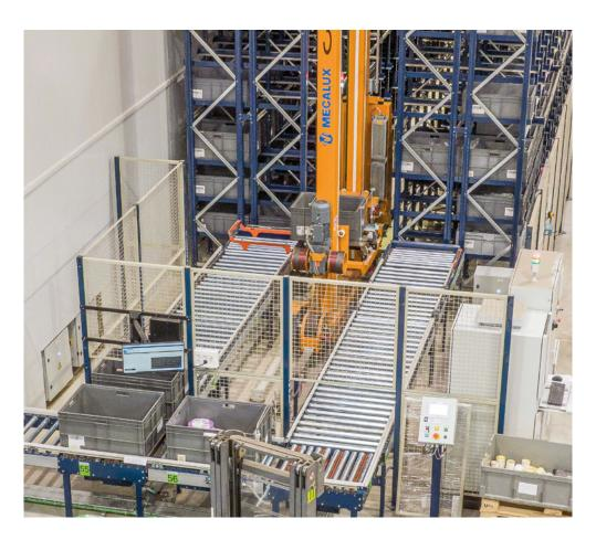
Meanwhile, in the automated installation, pallets have to go through a checkpoint, where their sizes are verified. If the measurements fall within the corresponding ranges, Easy WMS directs the stacker cranes to place the pallets in their assigned locations.
