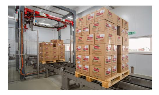
Mecalux proposed installing the automatic version of the Pallet Shuttle system with stacker crane because it combines all the advantages of high-density storage and automation. This solution is the result of merging the storage capacity of high-density systems with the reduction in the time spent on each operation, typical of automated systems.
