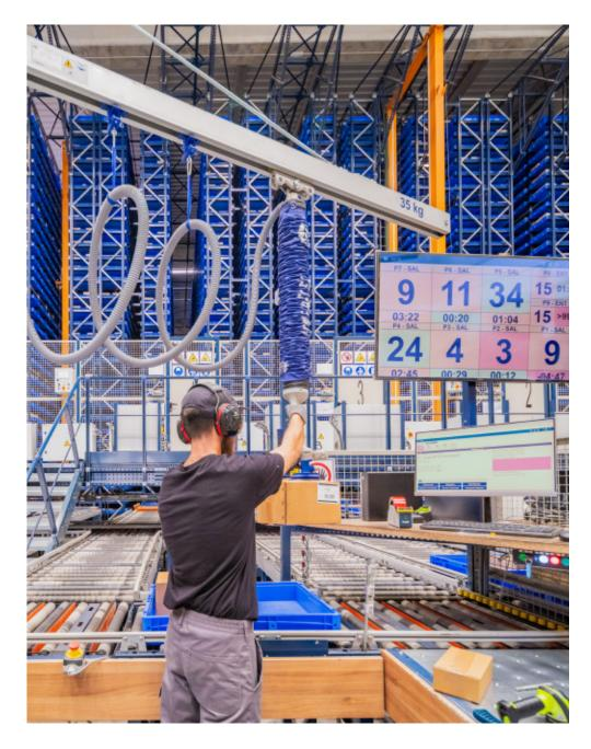
The station's two mechanical handling arms enable operators to work ergonomically. The bins are subsequently placed onto a conveyor system, which transports them to the automated warehouse. A lift bridges the difference in height between the two facilities.
