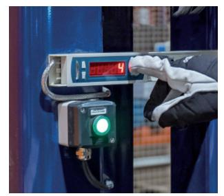
The put-to-light device shows the number of SKUs to place on each pallet. Once the process has been completed, the operator presses the button to validate their picking. This system provides high operational agility, reduces errors in order fulfillment, and enables real-time stock updates by transmitting all information to the WMS.
