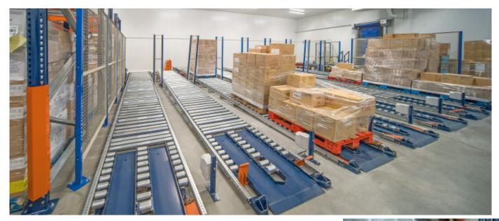
Goods kept safe: The shipping area also works at a controlled temperature to not break the cold chain. Additionally, retainers, brake rollers, and other devices installed in the preload channels automatically control pallet speeds and stops, without jamming or collisions.
