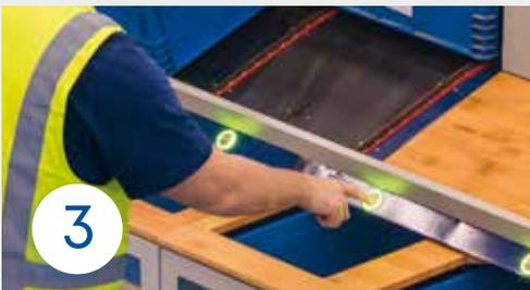
3 **Put-to-light and pick-to-light** systems provide associates with additional information on how to complete orders.
