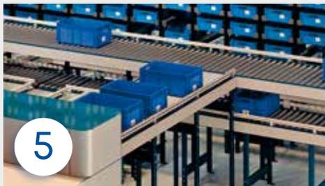
5 When the order is completed, the **tote on the lower level moves to the consolidation area**, and an empty tote takes its place to fill a new order.
