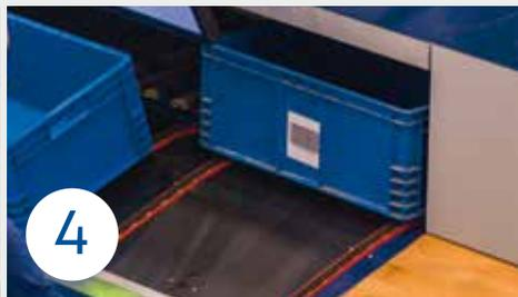
4 Once all the necessary products have been retrieved, the associate presses the confirm button, and the **bins on the pick station's upper level return to the warehouse.**
