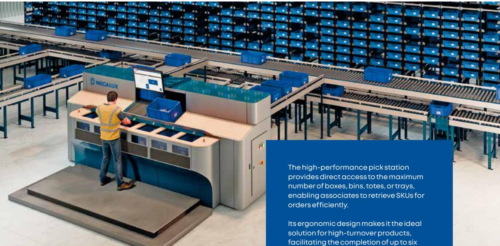
The high-performance pick station provides direct access to the maximum number of boxes, bins, totes, or trays, enabling associates to retrieve SKUs for orders efficiently.
