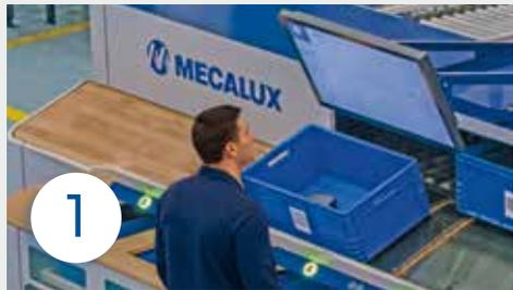
1 The **associate checks the instructions** from the Easy WMS warehouse management system on the screen, which displays the items and quantities to retrieve from each bin.
