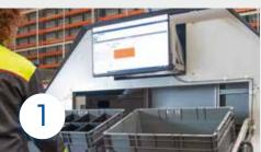
The associate checks the instructions from the Easy WMS warehouse management system on the screen, which displays the items and quantities to retrieve from each bin.
