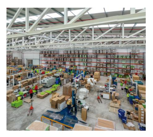
storage area has been leveraged by narrowing the working aisles to the fullest extent. This has enabled the firm to maximize storage capacity in the smallest possible area. Francisco Martínez Piedras can store 6,606 pallets and access them all directly, thus facilitating goods flows and order prep.
