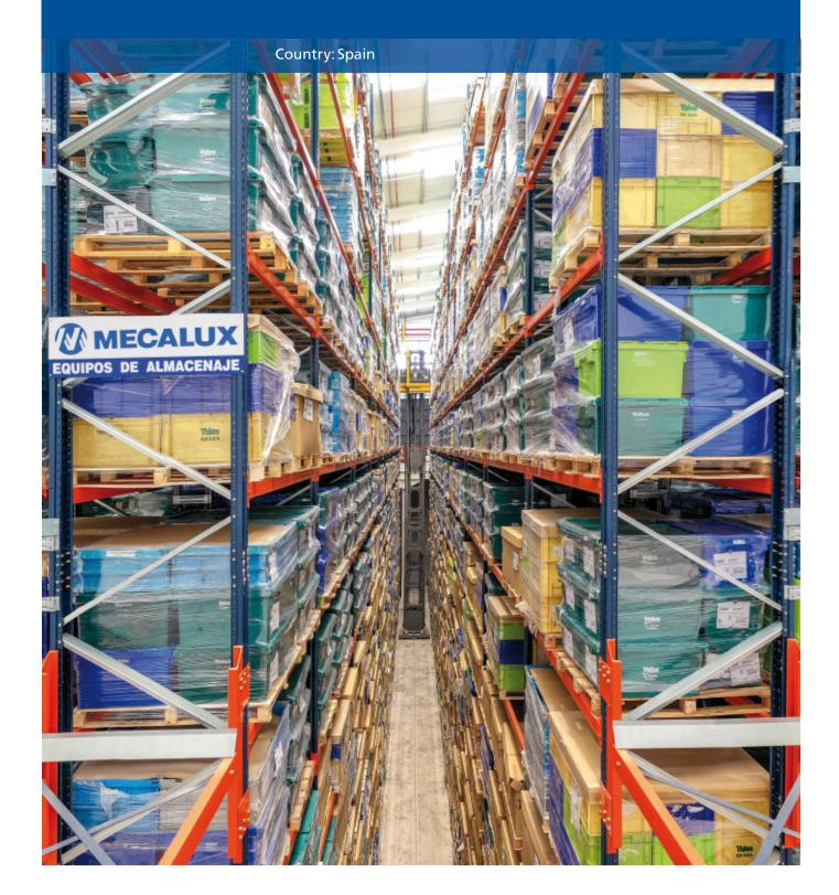
Francisco Martínez Piedras has centralized its logistics operations in two warehouses located next to its plant in Martos (southern Spain). Both have been equipped with narrow-aisle racks measuring up to 62' tall, thus optimizing both the surface area and height of the installation. Every day, a total of 7,500 SKUs are managed, while 18,000 car parts are dispatched in 1,200 pallets, which are then distributed to the company's customers in Europe, China and the US.
