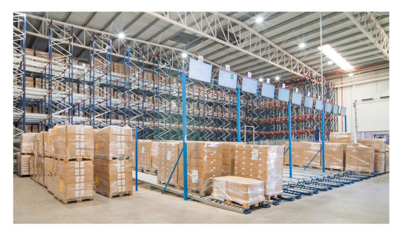
the trucks' load volume, a pallet placing device that stacks one pallet on top of the other has been set up. A transfer car has also been installed. This sorts the pallets into 11 flow preload channels based on whether they correspond to the same order or transportation route.
