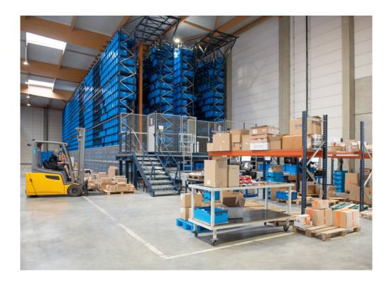
The AS/RS for boxes has doubled picking throughput compared to manual storage systems
