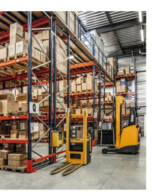
with Movirack mobile racks to hold an additional 1,120 pallets.
