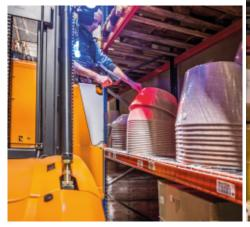
Racks with narrow aisles optimize the available warehouse surface in order to obtain a larger storage capacity
