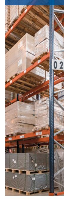
The two new warehouses that Leroy Merlin has constructed in Torija (Spain) are composed of pallet racking from Mecalux. Overall, they offer a warehousing capacity that exceeds 21,600 pallets. As a system that stands out for its versatility to house different size and volume pallets, it also yields highly-agile storage work.
