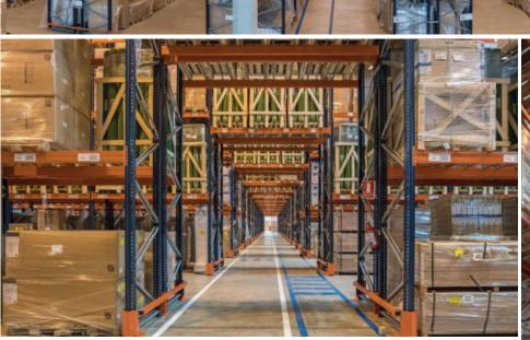
Operators work via zones and are assigned to a few working aisles. They use forklifts to insert and extract pallets from their corresponding locations.
