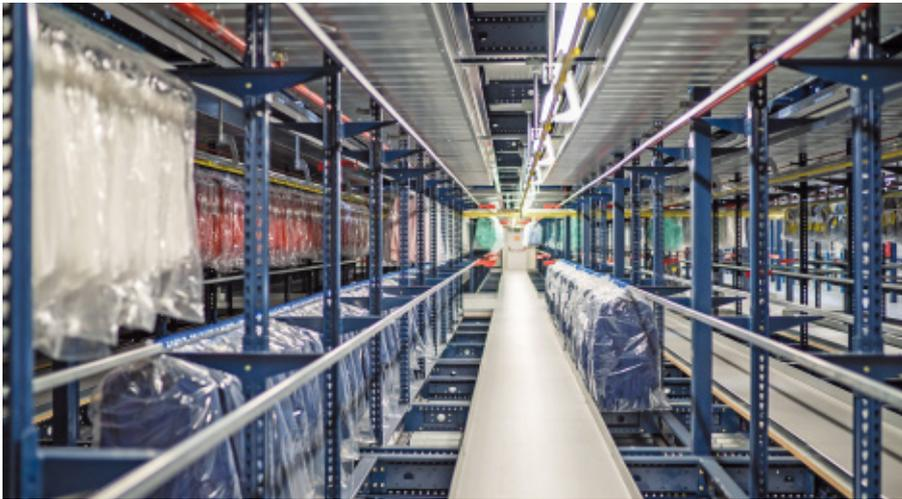
The tubes used for hanging garments on the racks are located at an optimum height from an ergonomic point of view. Although they have bearings every 7.2', the hangers slide and are grouped by SKU without producing any interference.
