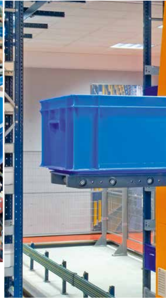
Extraction system with forks to extract two boxes at the same time
