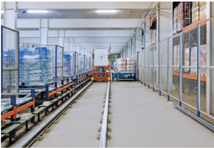
In this example, pallets from production move toward outgoing channels, with the transfer car in charge of linking the different origin channels to the destination ones.
