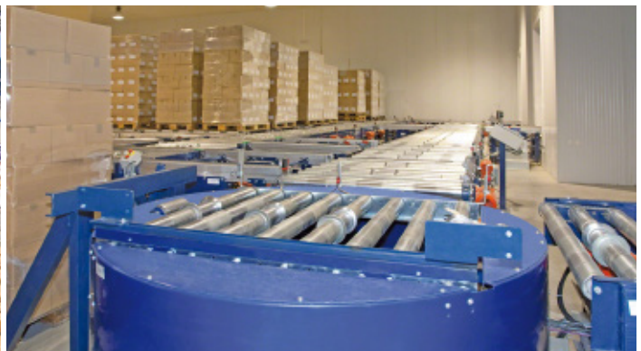
Mixed transfer with rollers and chains
