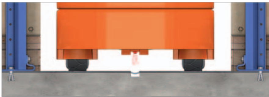
Wire-guided guidance A wire embedded in the floor produces the magnetic field that guides the forklift.
