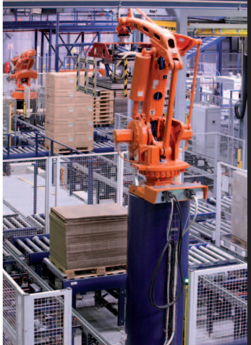
Automatic picking system depalletizer robot operation outline.
