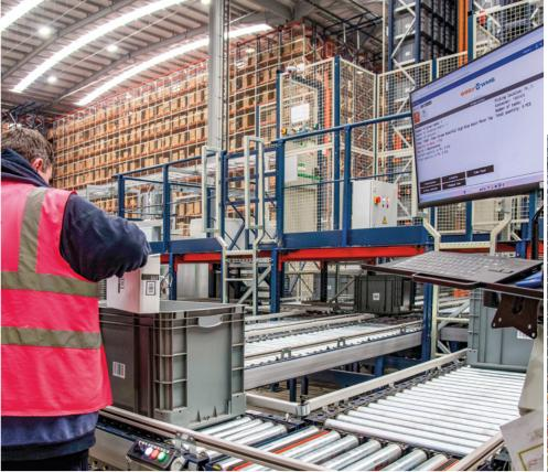
To speed up order fulfillment, conveyors automatically transport pallets and totes containing all types of bathroom items and accessories to the pick stations
