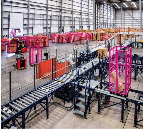
Products are placed in cages on pallets to prevent items from falling and eliminate the need for constant stretch wrapping
