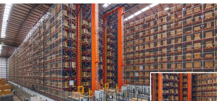
Smaller items, including faucets and bathroom accessories, are housed in a 39.4' high mini-load AS/RS for 7,900 totes. "We've seen a significant improvement compared to our previous manual operations. The system's ability to swiftly and reliably supply the picking area has increased accuracy and reduced errors," says Bacon. To further enhance fulfillment performance, a put-tolight system was installed on shelves located just behind the two pick stations.
