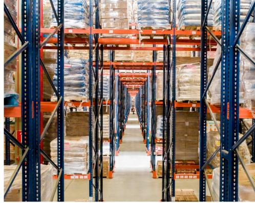
These occupy almost the entire surface area and facilitate goods management. On a normal working day, the operators walk through the storage aisles introducing and removing pallets from their corresponding locations using reach trucks.
