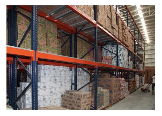
Mixing and matching single- and double-depth racks mean SKUs can be organized according to their features and demand level. In the words of Álvarez Mendoza, "Double-deep pallet racks were chosen because they entail a space savings that requires fewer aisles to access the loads. Plus, this solution ensures maximum storage capacity."
