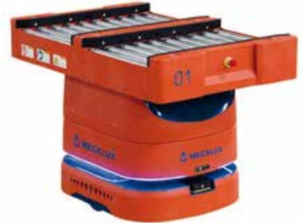
AMR 100 box with **double side load** conveyor with parallel transfer for 15.7" wide boxes.
