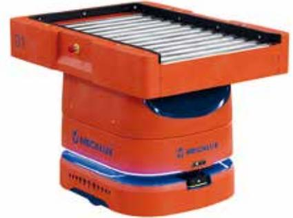
AMR 100 Box with **double front load** conveyor with in-line transfer for 23.6" wide boxes.
