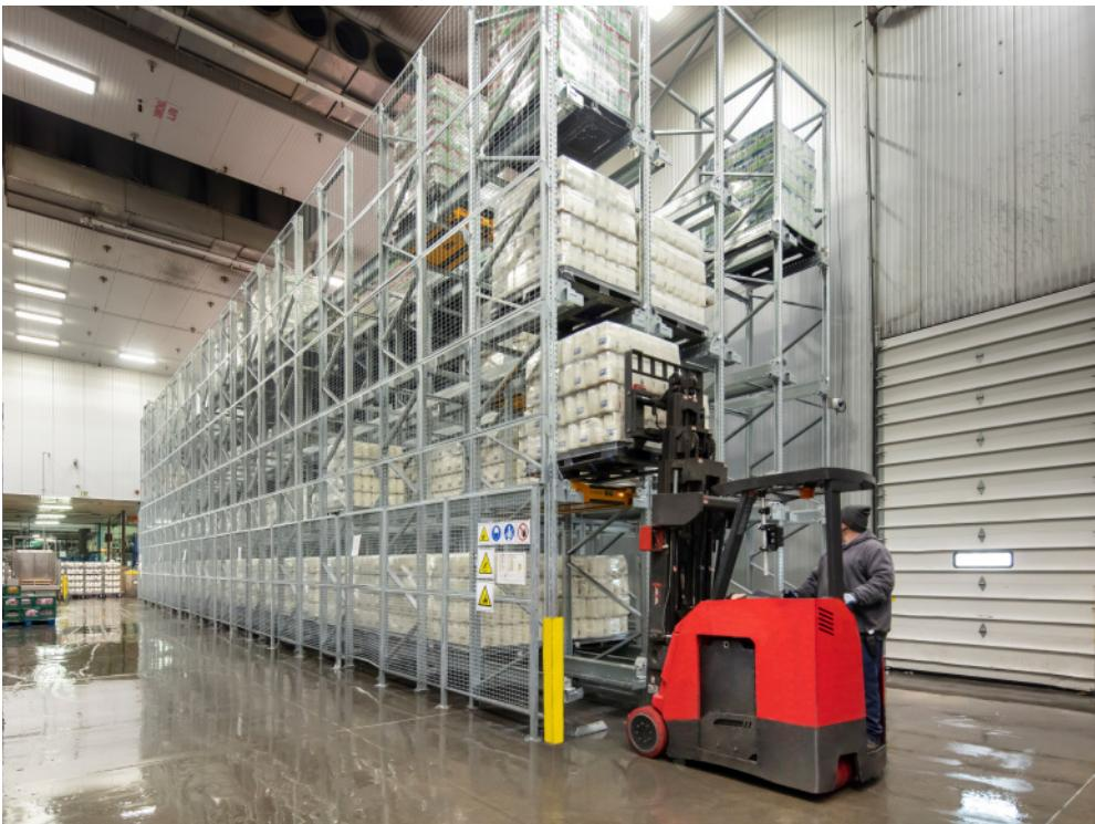
**The high-density, semi-automated system uses a shuttle that runs along rails inside a storage channel**
