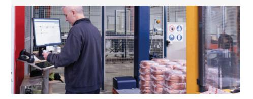
WMS checks whether the reel containing the cable matches the one requested by the customer. If it does, it is brought directly to the consolidation zone. If it does not, the reel is changed at one of the cutting stations.
