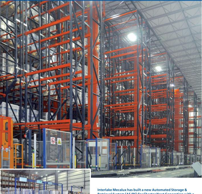
Interlake Mecalux has built a new Automated Storage & Retrieval System (AS/RS) for Charter Next Generation with a storage capacity for more than 15,400 pallets of different sizes and turnovers. The installation is managed by the efficient Easy WMS warehouse management system by Mecalux, capable of maximizing the productivity of all operations being performed.
