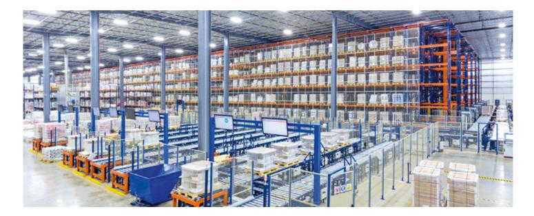
With these factors in mind, only an internationally recognized and experienced firm like Interlake Mecalux could construct the ideal warehouse that would efficiently fulfill Charter Next Generation' requisites. After an in-depth study, Interlake Mecalux proposed the construction of a 39' high AS/RS for pallets installation inside the Charter Next Generation premises. It comprises six aisles with double-depth selective racks on both sides, whose storage capacity exceeds 15,400 pallets.
