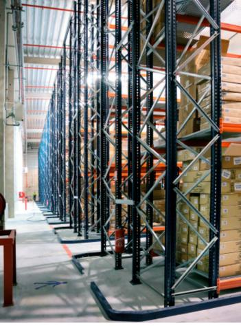
Long span mesh shelves allow for an increased storage capacity and let the operator step up onto the shelf to reach the boxes located in the second and third positions
