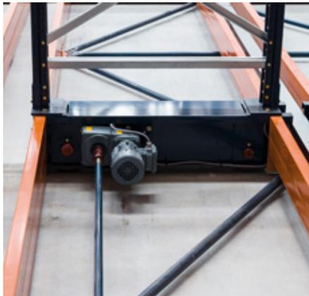
The transmission of power to the mobile base is undertaken through a double crown gear with a double pinion, which provides better system performance. By doing so, this ensures that the movement of the racks is more uniform and, therefore, the life of the mechanical components is extended.
