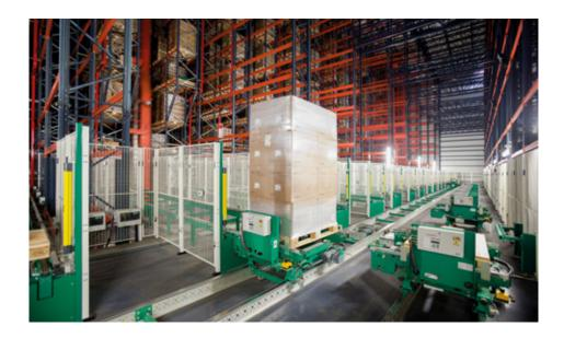
Autonomous trolleys, circulating via electrified monorails, connect the aisle input and output conveyors with warehouse outbuildings, where the tasks of receiving, sorting and forwarding of orders are performed
