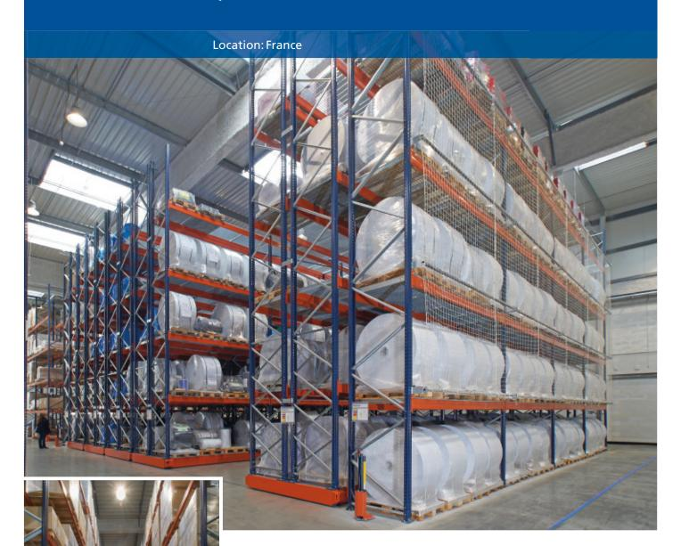
Mecalux has supplied Cartolux-Thiers with pallet racking to deposit completed orders on and Moviracks on mobile bases allocated to the raw materials needed in their production process. With the combination of these solutions, the company who manufactures thermoformed packaging has obtained a storage capacity of more than 2,800 pallets.
