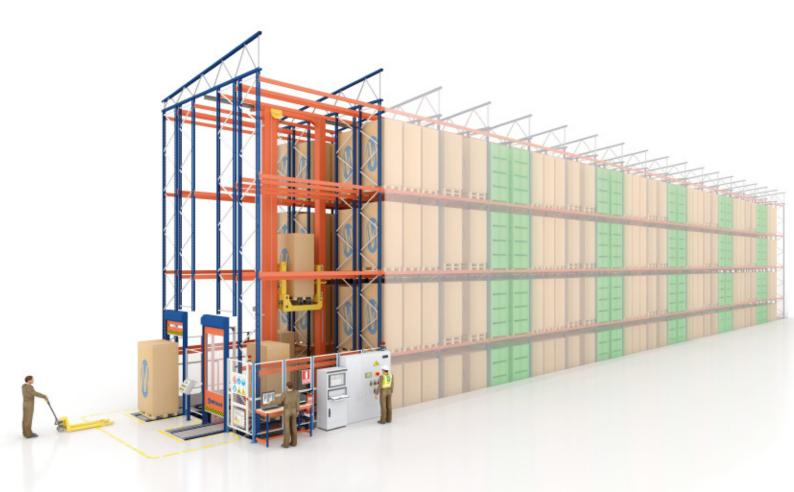
The racking, divided into four levels, has been personalized to be able to accommodate three different unit loads: 47" x 47" plastic containers and pallets measuring 32" x 47" and 39" x 47". In the case of plastic containers, each location can store up to four containers stacked one on top of the other.
