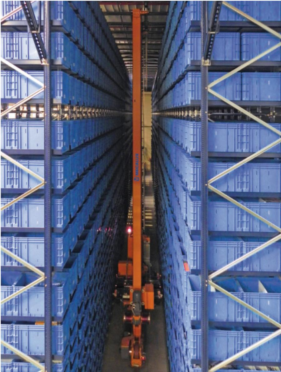
analyzing its requirements, Mecalux proposed building an automated warehouse with capacity for 6,000 boxes with about 6,500 SKUs. In just 3,230 ft<sup>2</sup> of surface area, the automated facility is capable of managing the same SKUs that used to be stored on a 16,000 ft<sup>2</sup> mezzanine floor.
