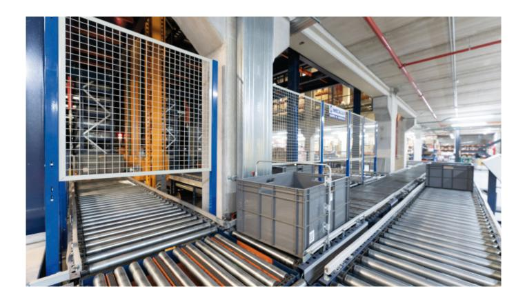
ual picking zones, are sent to an area comprising 17 flow conveyor channels. Boxes that make up a single order are placed in one of the channels and then moved to one of the four packing and labeling stations.
