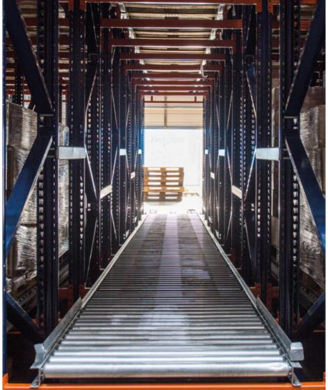
On the bottom level of the racks, pallet flow channels make product classification by order or route possible, and thus streamlined loading of distribution trucks
