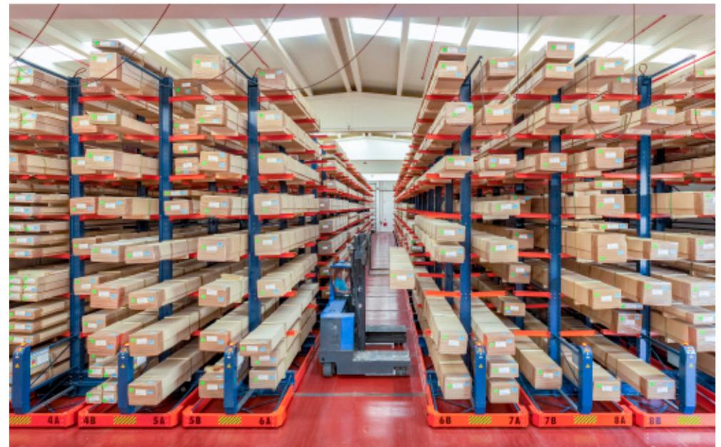
tures with wheels — activated by integrated motors — that move along rails.
