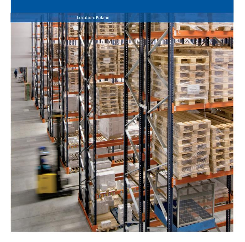
Ziaja, Polish manufacturer of natural cosmetics and pharmaceuticals, has a new warehouse designed specifically to streamline picking, the chief operation of the center. Mecalux has installed standard pallet racking, which offers direct access to the goods and has a storage capacity of 10,906 pallets.
