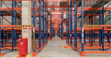
Mecalux has equipped the Unilever warehouse in Brazil with both single and double-deep pallet racking, providing an 83,569 pallet storage capacity. With this solution, the company can meet its customers' demand for products and enhance the growth rate achieved in Latin America.
