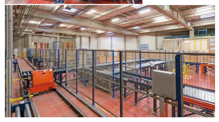
The conveyor circuit also incorporates a full pallet stacker, which can lift the pallets to place them on slave pallets, and a station where empty pallets are stacked and unstacked.
