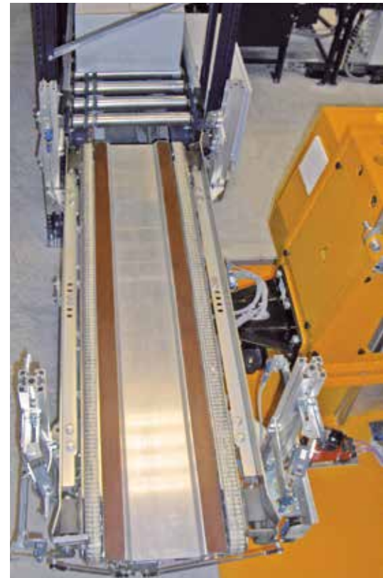
Details of the extraction system that combines forks with belts (EC).
