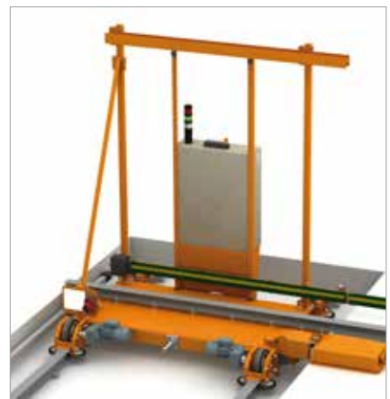
Details of a transfer bridge (2).
