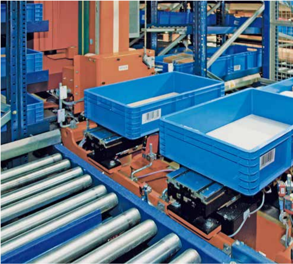
Extraction system with forks to extract two boxes at the same time
