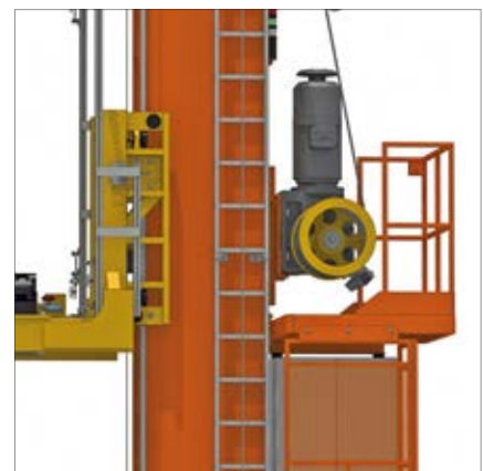
Hand ladder and top maintenance platform
