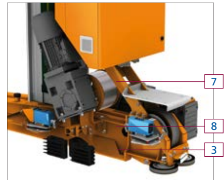
Lower guide base (3), lifting components (7), and rangefinder (8)
