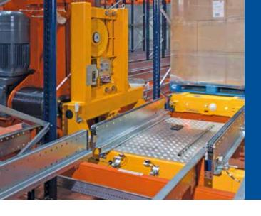
The automated Pallet Shuttle is a compact storage system that uses electric shuttles and automated handling equipment (stacker cranes or transfer cars) to boost the capacity and productivity of the warehouse. The system executes the orders given by the Easy WMS warehouse management software.
