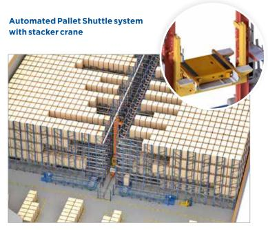
The stacker crane executes movements from the AS/RS input and output positions to any storage channel. The pallet shuttle is tasked with moving the pallets from the cradle of the stacker crane to the location in the corresponding channel. Generally, two compact storage racking units are installed, one on each side of the working aisle.
