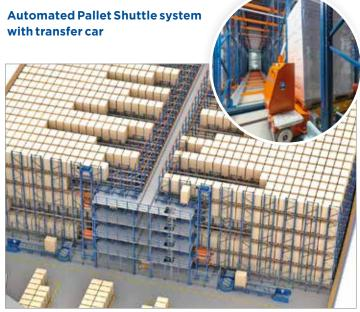
Instead of a stacker crane attending to all levels of all the storage channels, a walkway-type structure is set up to enable a transfer car to move on each level. So, if the AS/RS is five levels high, five transfer cars are used to perform the movements from the lift to the storage channels on each level. This way, the number of movements (i.e., cycles/hour) is multiplied by the number of levels in the AS/RS.
